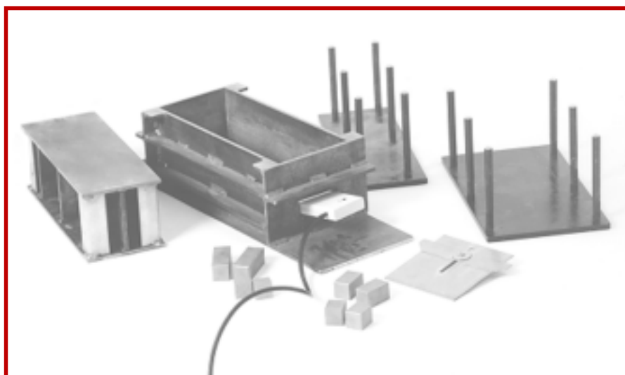
Figure 2c—Components used to prepare and remove soil samples from the mold.
