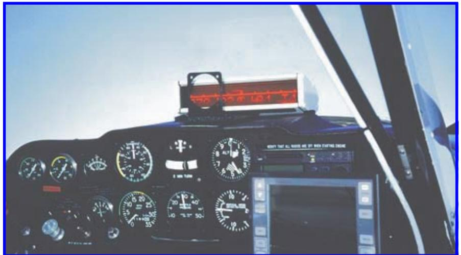
Cockpit-mounted DGPS aircraft guidance system.
