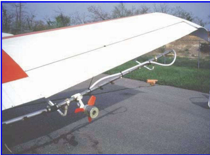
*Wing-mounted spray system for pheromone application.*
