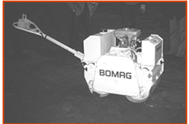
Figure 28—This Bomag walk-behind vibratory roller provides excellent compaction but is slow.
