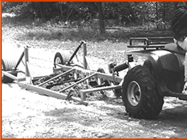
Figure 13—The Ultra Light Terrain Grader was designed for roads and parking lots. It works best there.
