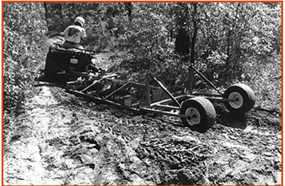
Figure 11—Due to its length and width, the Ultra Light Terrain Grader had a hard time negotiating corners.
