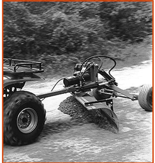
Figure 5—With two passes, the trail rake could pull in berm material from both sides to the center of the trail or road. Here, the scraping blade is being used.
