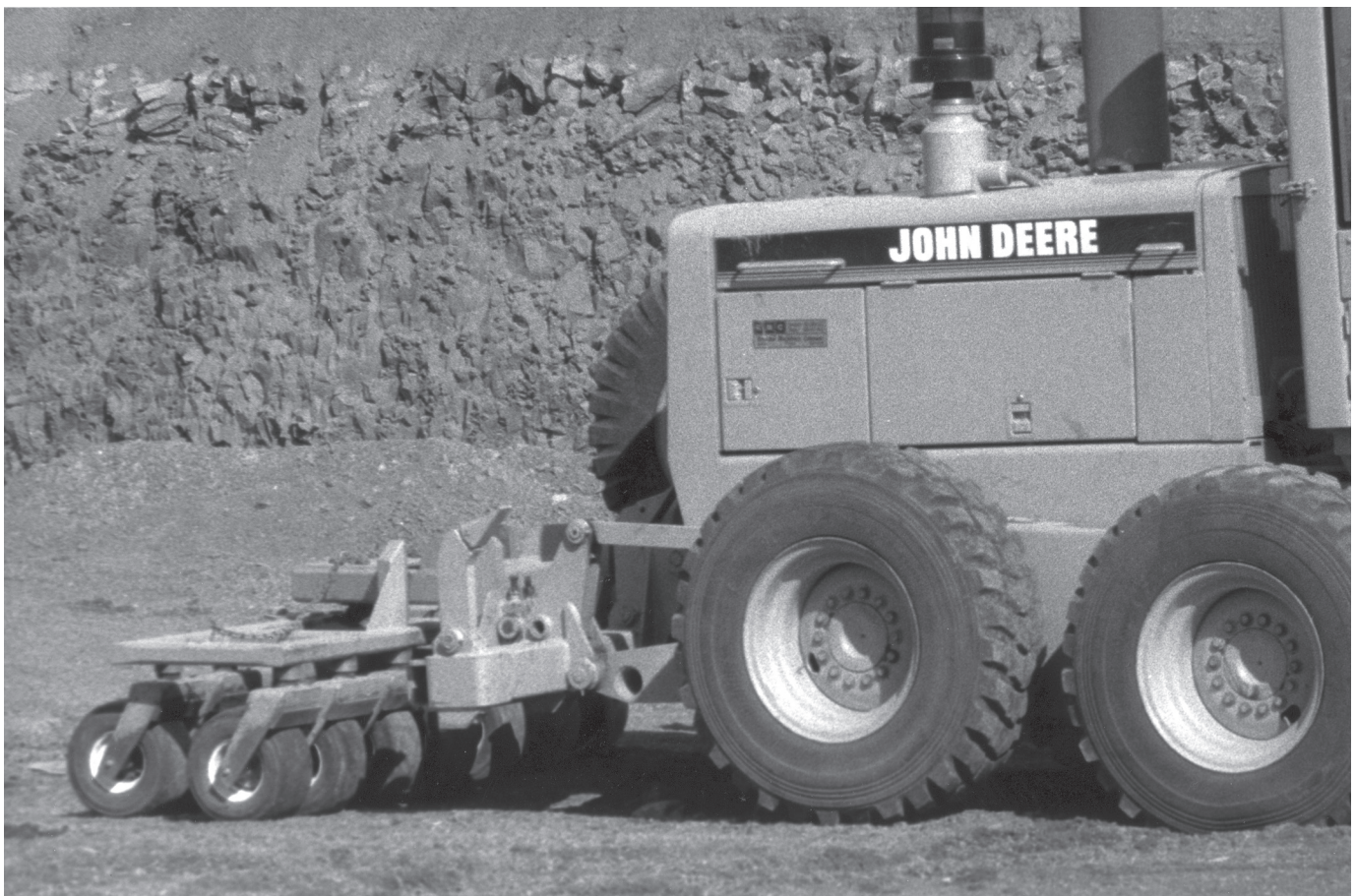
Figure 1—The modified compaction roller attached to the grader's toolbar maintains a constant pressure despite dips and rises in the road's surface.
