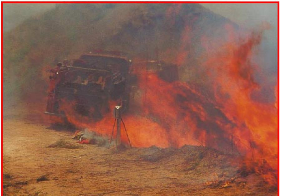
Figure 26—When a fire comes up a steep sideslope, it appears to go over and under the engine, creating an eddy on the back side that draws heat and flame.
