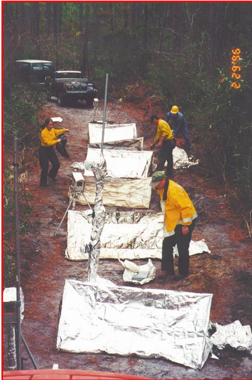
Figure 4—Several types of fire shelters were tested, including the standard Forest Service fire shelter and prototypes from MTDC and a private firm.
