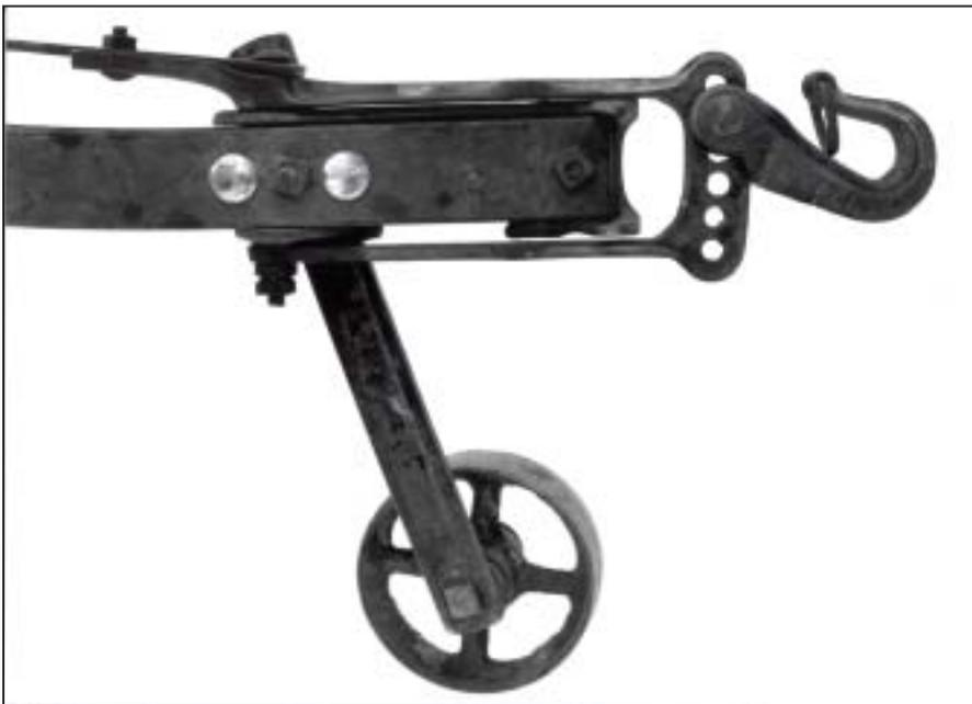
Figure 3—Vertical draft adjustment.
