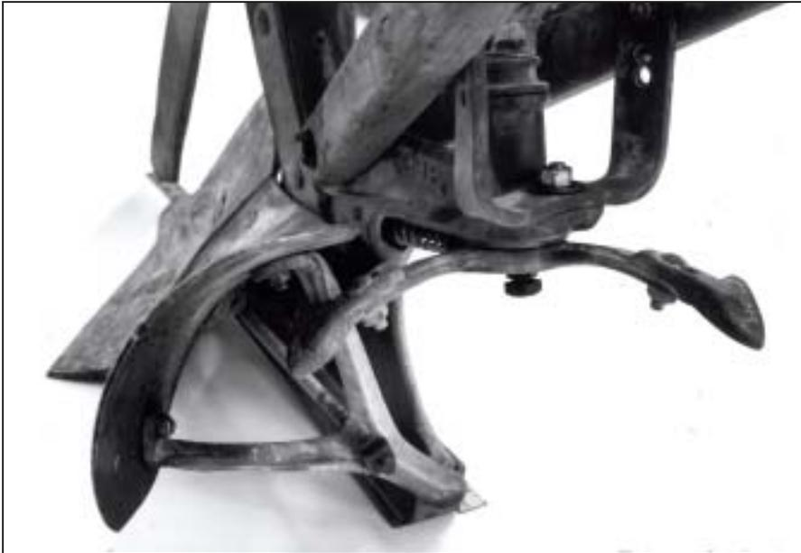
Figure 2—The latch on a hillside plow.
