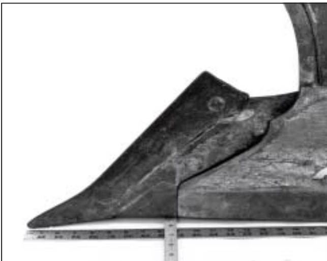
Figure 11—Oliver plow showing about  $\frac{3}{4}$  inch of bottom suction.
