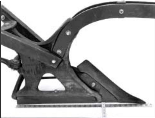
Figure 6—Vulcan plow showing about 1½ inch of hillside suction.
