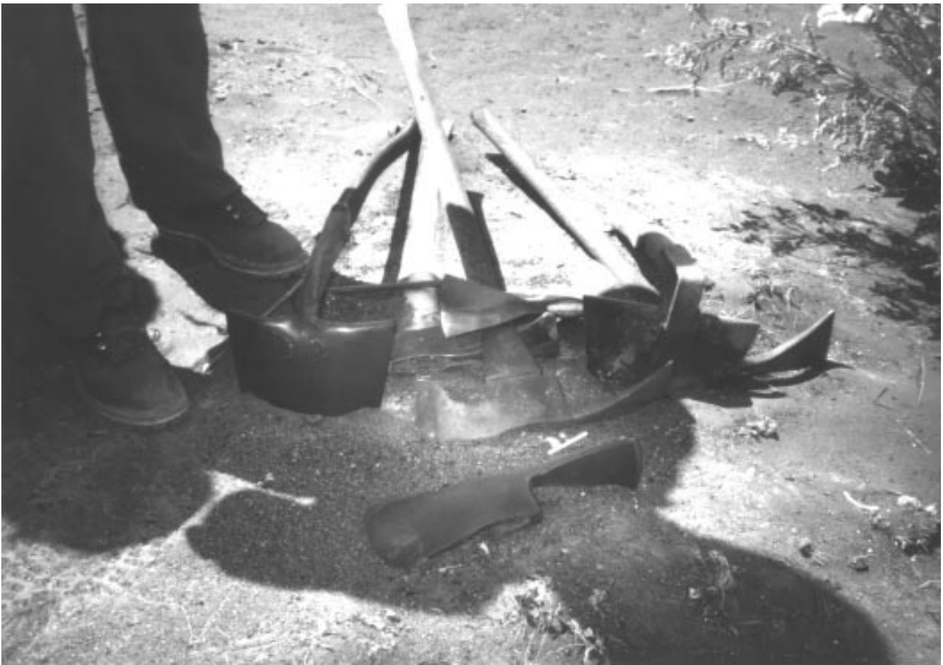
Inspection of fire damaged equipment and tools shows the range of heat exposure.
