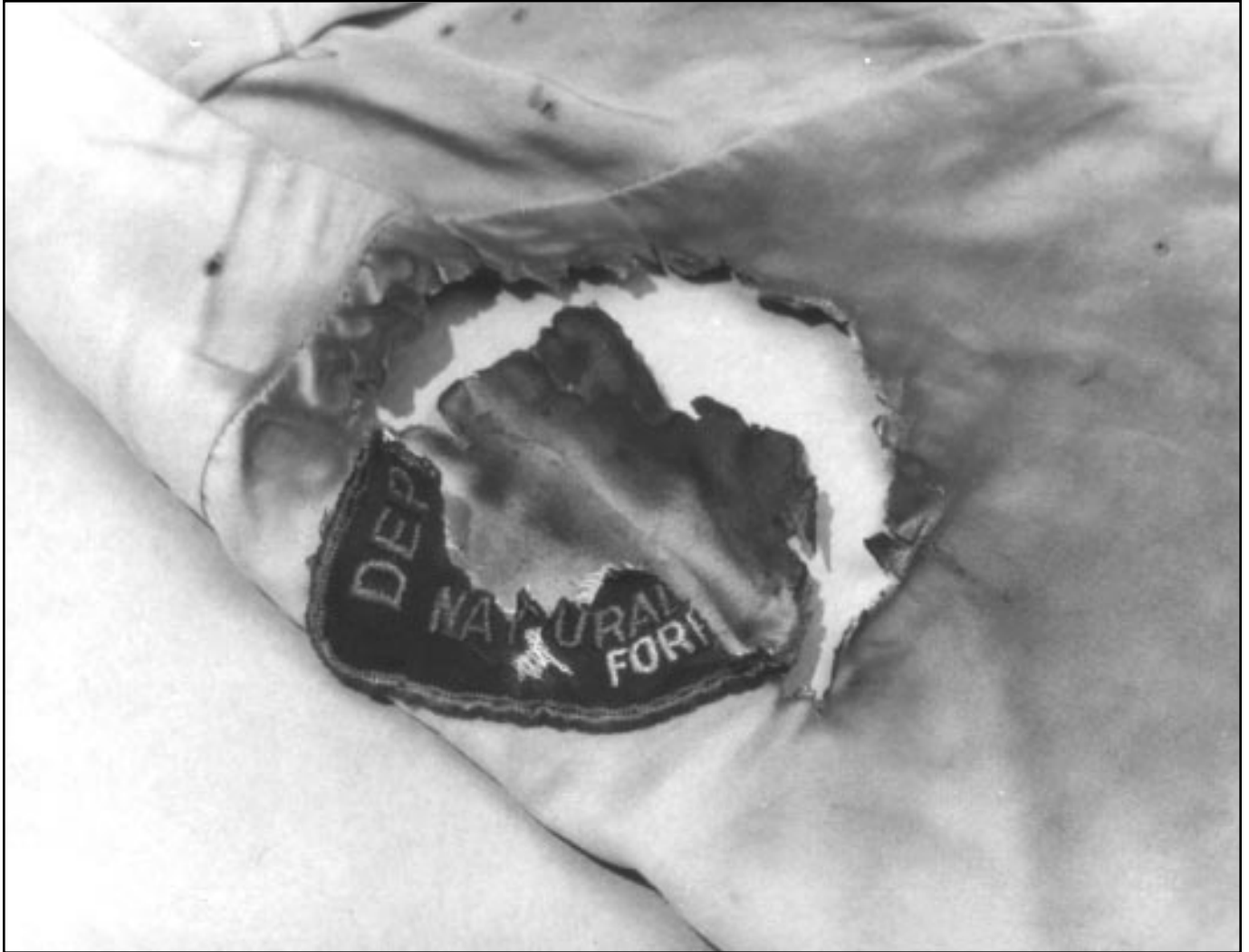
Fire-damaged personal protective clothing.
