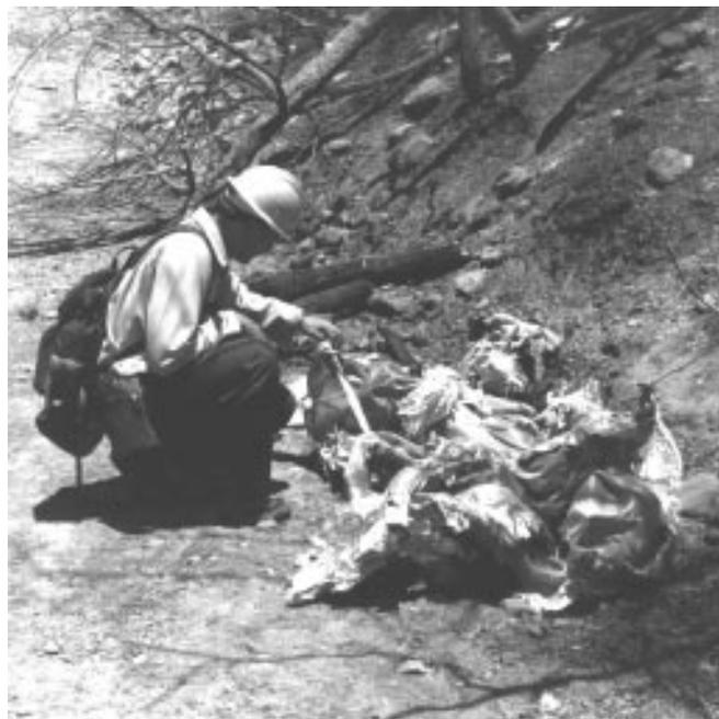
Close inspection of the fire shelter provides clues of temperature ranges during the entrapment.
