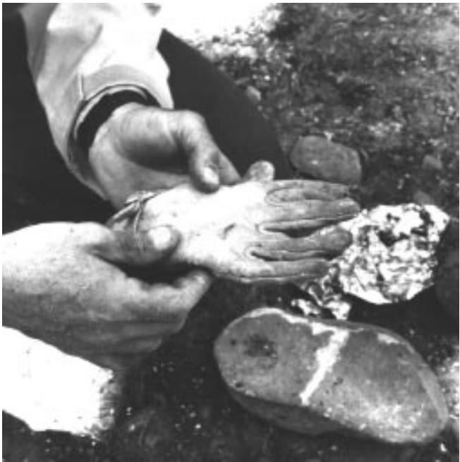
Firefighter's glove shows high temperature effects.
