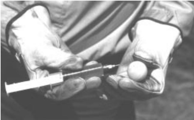
Figure 16.—Injecting the plastic sphere with potassium permanganate.
