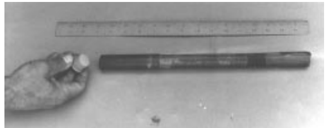
Figure 15.—Plastic bore sealing cap for fusees.
