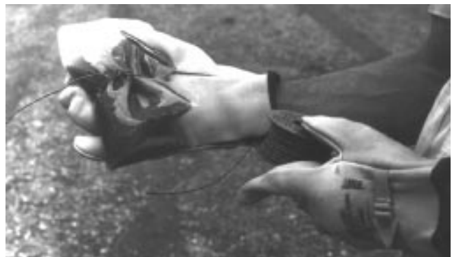
Figure 7.—Gelled gas inside bag, with an outward-burning fuse.
