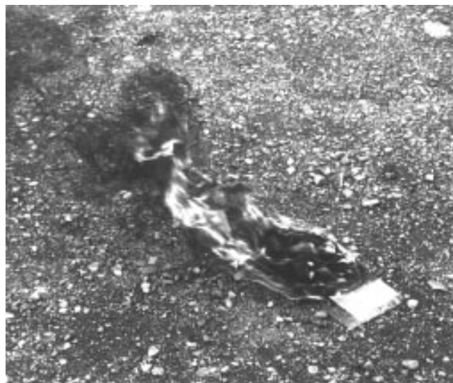
Figure 8.—Gelled gas burning inside bag.
