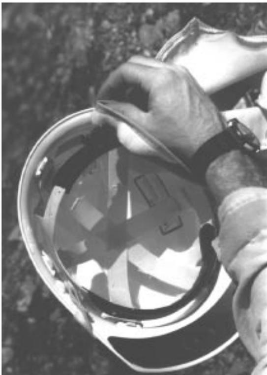
When not in use, the face/neck shroud can be rolled up and stowed between the hardhat shell and liner, or detached and kept in your pack.
