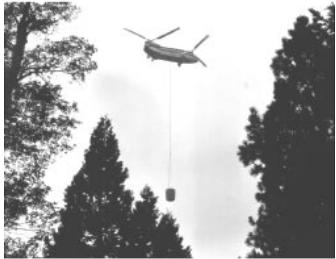
Flight time for heavy lift helicopters can be reduced if specific drop spots are coordinated between air and ground.
