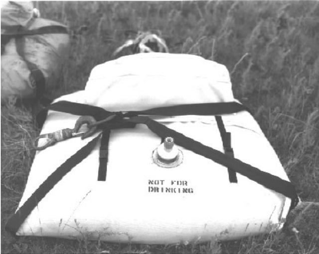
The suppression water bag is made of heavy nylon duck to ensure its durability.
