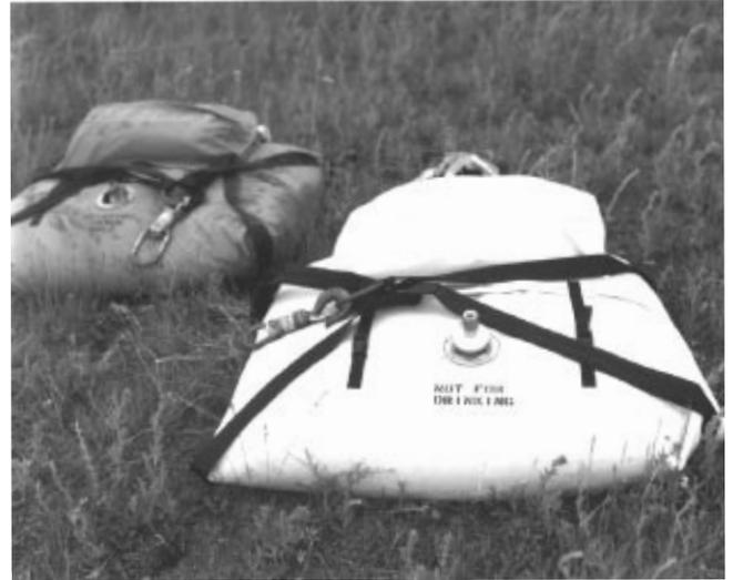
The 55-gallon water bags, prepared for slingload transport by helicopter. NOTE: The necessary swivel hooks have been attached to the o-rings (swivel hooks are NOT included with 55-gallon water bags).
