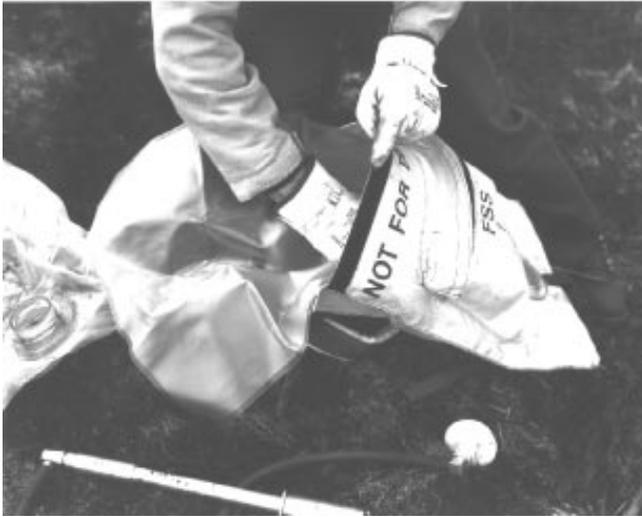
Replacing a suppression water bag liner in the field.
