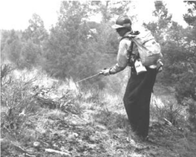
Comfortable and durable, the 5-gallon suppression water bag can be attached to the firefighter backpack harness.
