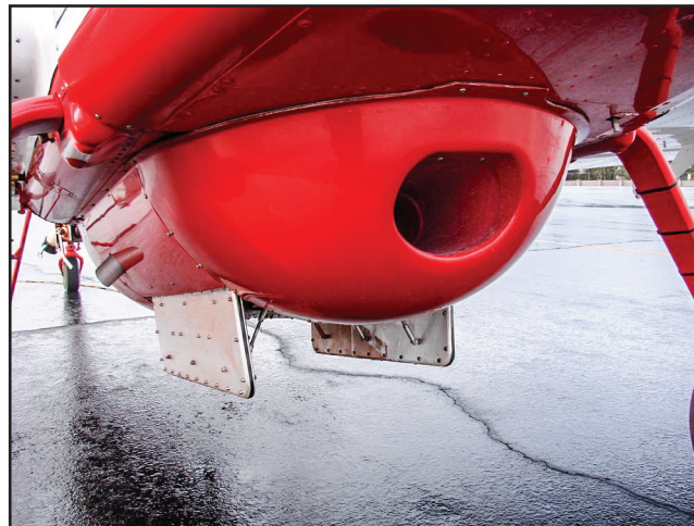
Figure 1—A Hydromax fire gate installed on an Air Tractor AT-802.
