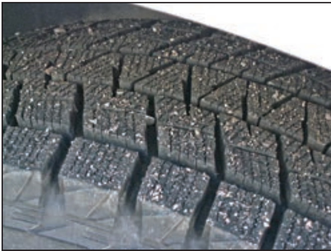
Figure 3—Studless tires employ various techniques to improve traction, such as this Bridgestone Blizzak tire that uses a special rubber compound with microscopic pores.
