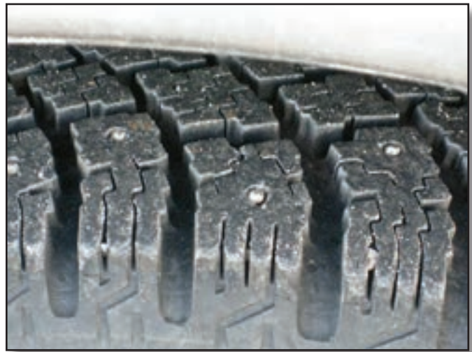
Figure 2—Studded tires may damage the road surface.
