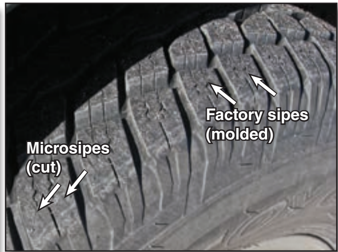
Figure 4—This tire has factory sipes and microsipes.
