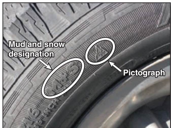
Figure 5—Tires designed for use in severe snow conditions are marked on at least one sidewall with the mud and snow designation and the pictograph.
