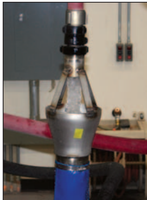
Figure 1—Testing the air gap prototype. The prototype, built by mechanical engineering technicians at the Missoula Technology and Development Center (MTDC), produces no splash while operating.
