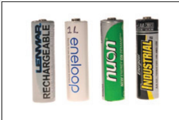
Figure 3—Three AA NiMH batteries (left) and one AA alkaline battery (right).
