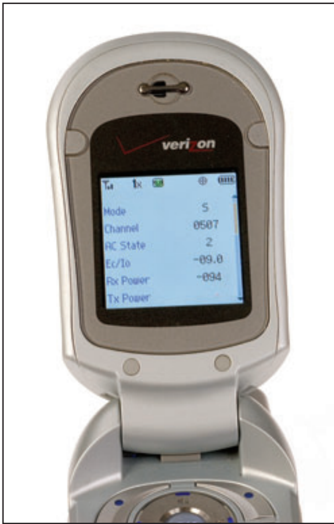
Figure 3—Diagnostic screens found on some cell phones offer a more accurate way of determining when a cell phone can complete transmissions than the bars most cell phones display.
