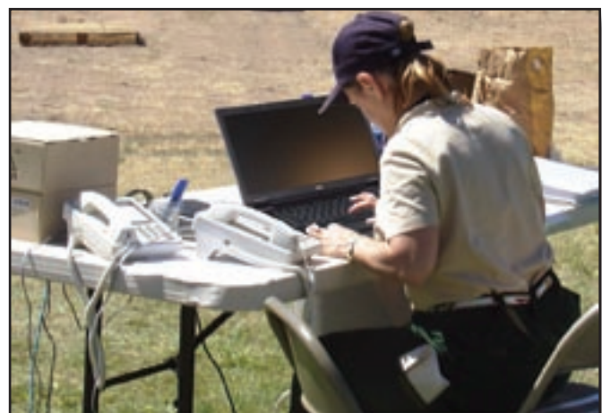
Figure 2—A mobile thin client (laptop without a hard drive) is used at an incident command post. The thin client allows users access to applications on the networking kit's server. During deployment testing, the mobile thin clients will use a wireless local area network (LAN).
