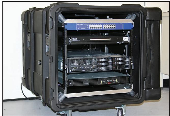
Figure 1—A terminal server is the heart of the thin client kit. The server and other hardware are mounted in a rugged case for protection. It will be transported and operated inside an air-conditioned trailer at the incident.
