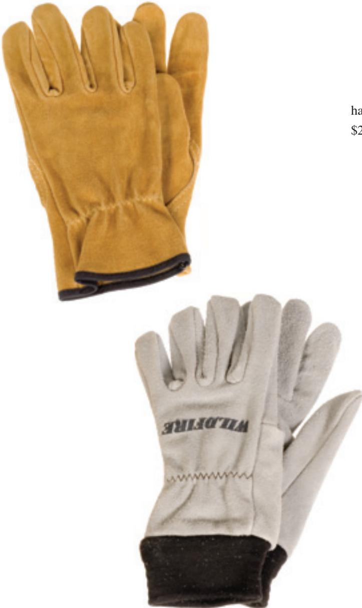
Both glove styles feature a gunn-cut design that has a single-piece seamless back with finer seams set farther away from the working area of the palm. The two middle fingers are sewn separately onto the palm piece. Gunn-cut gloves provide better wear and comfort, especially for heavier gloves. Both gloves have hanger loops to make them easier to carry.
