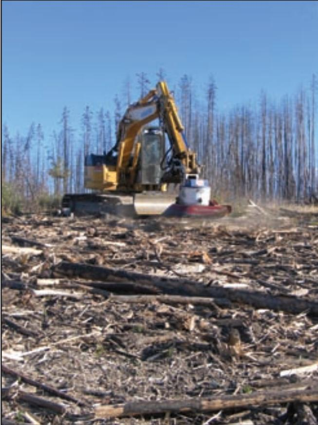
Figure 2—A Komatsu trackhoe with a slash-buster mechanical head and thumb attachments was used for rehabilitation.
