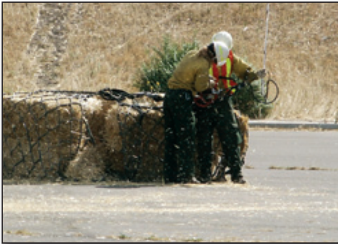
Figure 2—Attaching a loaded cargo net to the remotely controlled hook of a helicopter longline.
