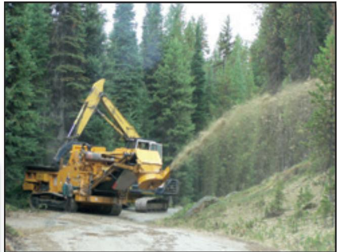
Figure 4—A horizontal shredder fed by a trackhoe can shoot shredded material into the woods for erosion control.
