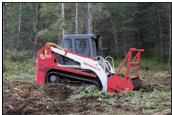
Figure 2—A mastication attachment on a small skidsteer.
