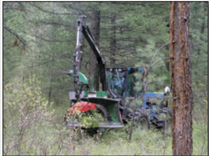
Figure 5—A self-feeding wood chipper attached to a tractor.
