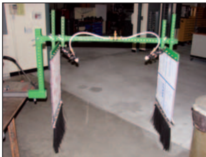
Figure 3—The new design allows both the nozzles and the shield to be adjusted, providing good spray coverage on weeds and grass while keeping overspray off desired crops.
