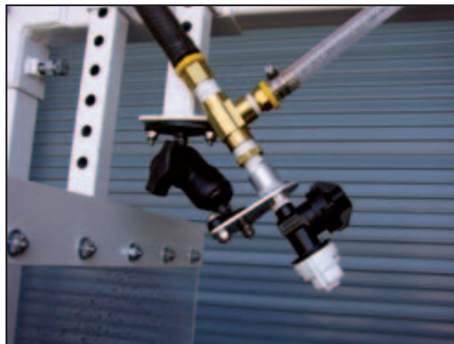
Figure 4—RAM mounts allow nozzles to be rotated and set at various angles to ensure herbicides are directed toward weeds and grasses and not onto bareroot seedlings nearby.
