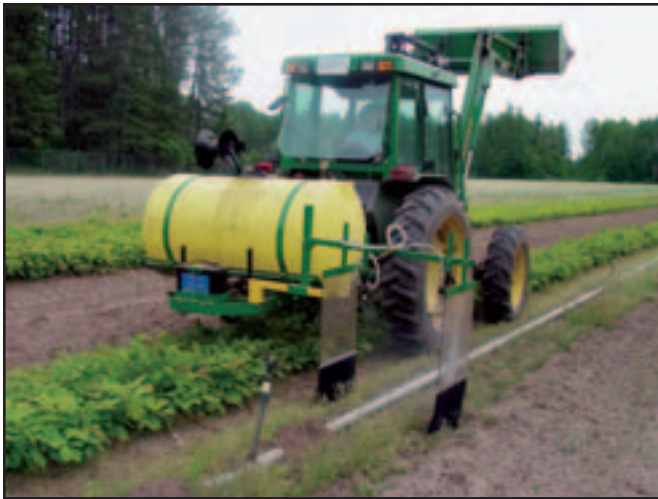
Figure 5—A sprayer shield assembly is shown mounted to a three-point hitch sprayer designed specifically for spraying around irrigation pipelines.
