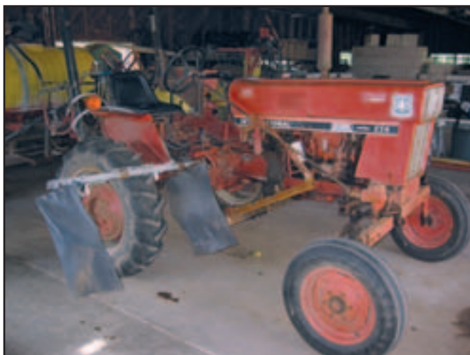
Figure 2—A pipeline spray shield is attached to the underbelly mount on an International tractor at the J.W. Toumey Nursery, Watersmeet, MI.
