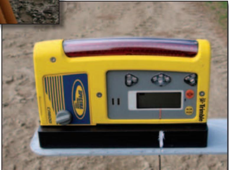
Figure 5—Both the AGL Laser Receiver MR360R (left) and the Spectra Precision Laser Receiver CR600 (right) can intercept a laser beam from more than 1,000 feet. Bright LED lights allow the display to be seen even in bright daylight.
