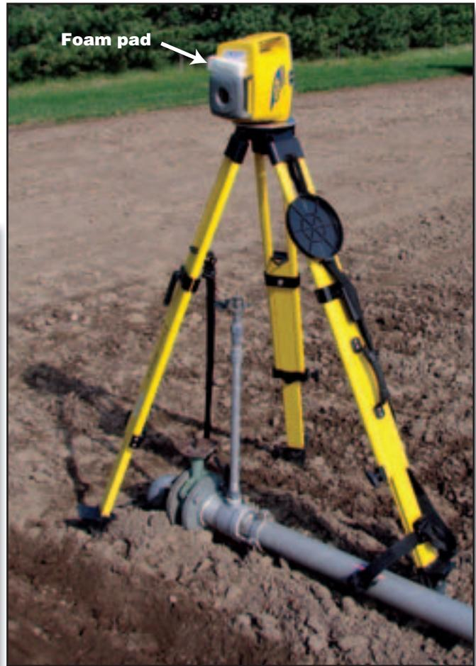
Figure 4—To help keep irrigation pipe in a straight line, the laser is centered and manually leveled over the irrigation pipeline's riser. The foam pad prevents the rotary laser's beam from being projected straight up where it could cause problems for aircraft pilots.
