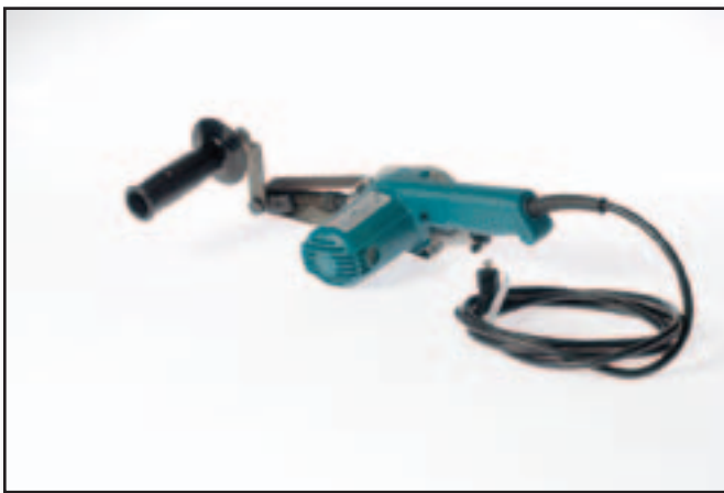
Figure 3—The commercial 1½ inch-wide belt sander (Makita Model 9031) used for sharpening.
