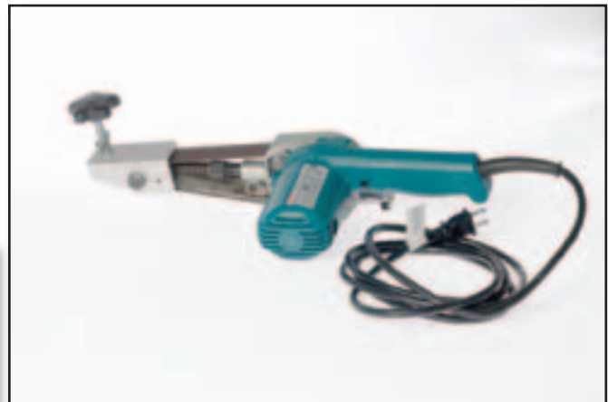
Figure 5—The new bracket attached to the narrow belt sander.
