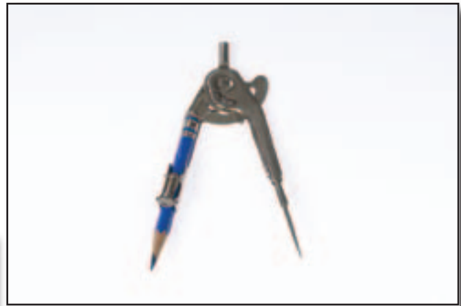
Figure 7—For some single-bit axes, a compass is used to determine the pivot point for a sander fitted with the new bracket.
