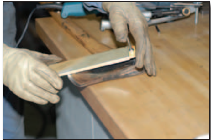
Figure 12—To finish the sharpening job, remove the blade's wire edge with a fine-grit diamond stone.
