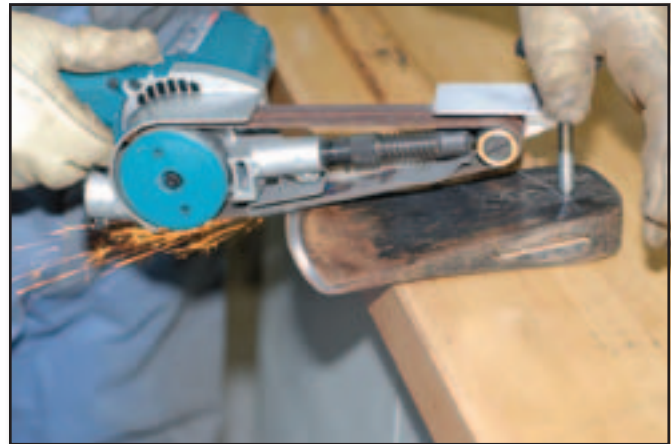
Figure 1—A newly developed bracket allows a narrow belt sander to be used much like a draw file for sharpening axes and Pulaskis.
