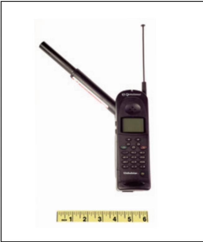
Figure 2—A satellite phone provides duplex (two-way) communication.
