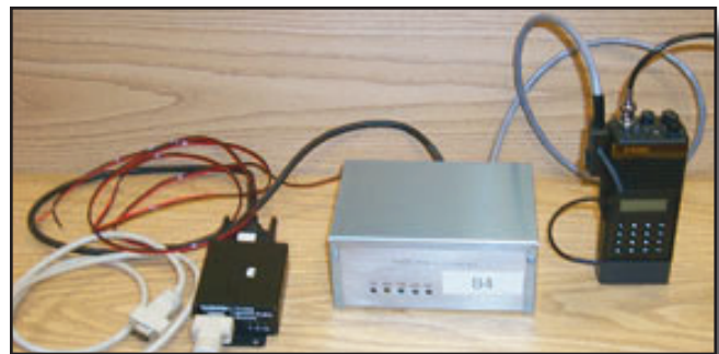
Figure 1—Data is transmitted from a remote site by a modem (left), interface (center), and Bendix-King radio (right).
