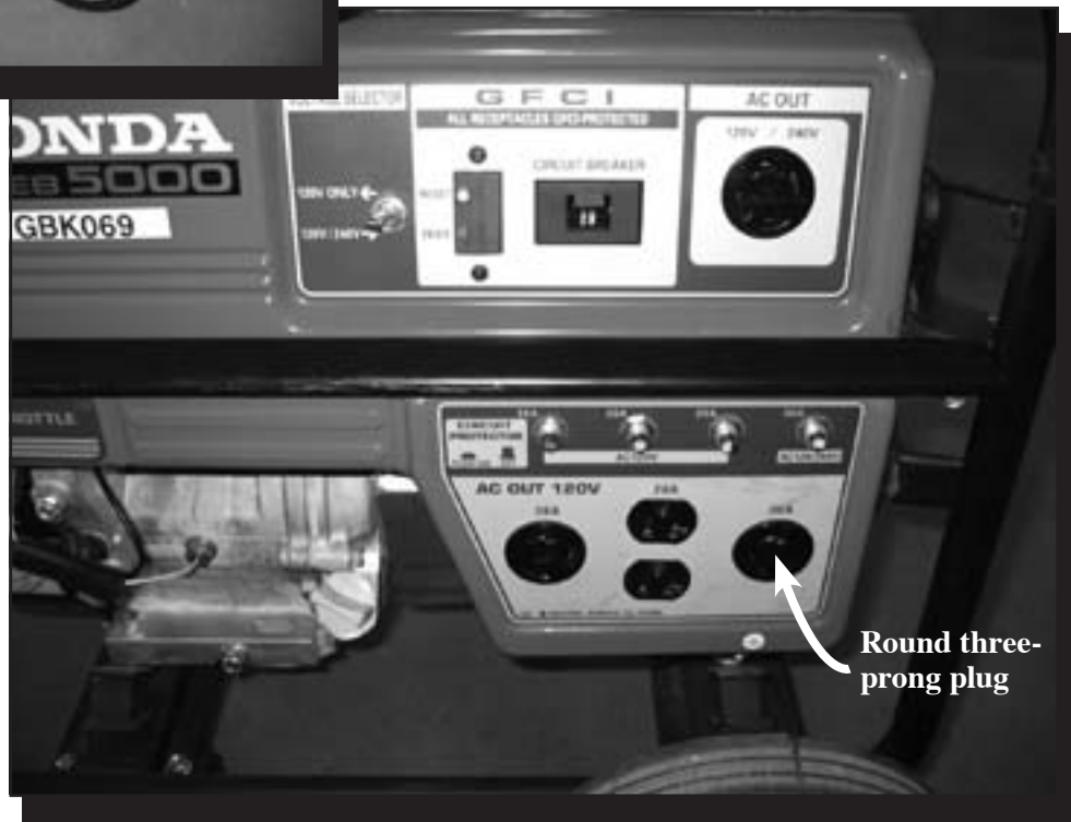
Figure 2—The control and outlet panel on a small portable generator.
