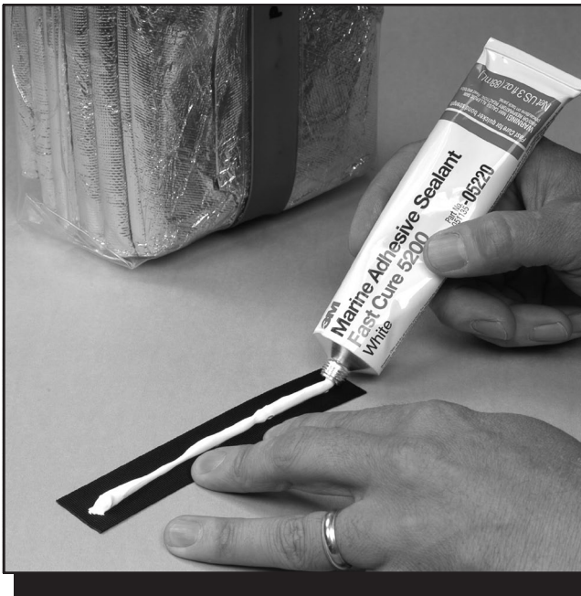
STEP 1: Apply a thin bead of adhesive to the nylon webbing.
