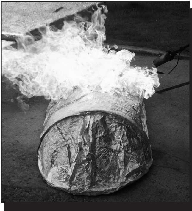
Figure 6—Flames are impinging on a New Generation fire shelter during a surface temperature test.
