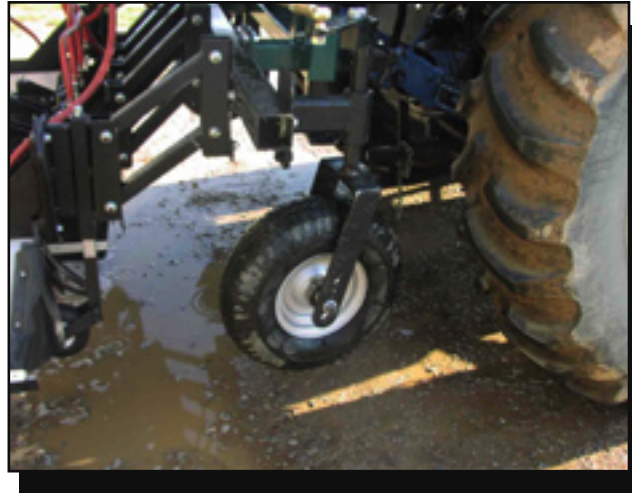
Figure 23—The improved version of the steering guide wheel on the MTDC Shielded Herbicide Sprayer.— Courtesy of the Virginia Department of Forestry
