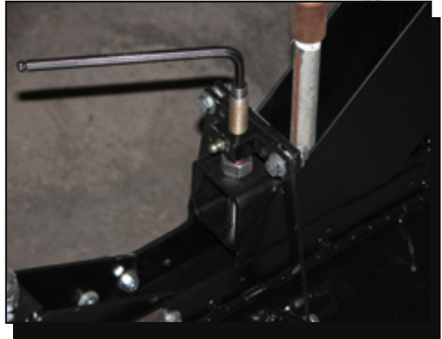
Figure 21—The mechanism used to adjust the width of a sprayer hood on the MTDC Shielded Herbicide Sprayer.
