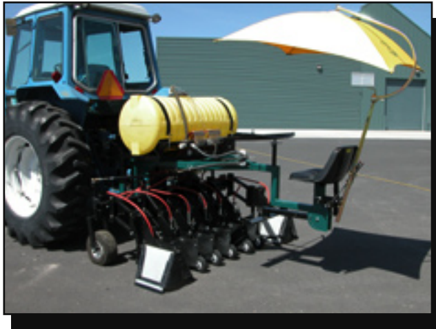
Figure 19—The second-generation MTDC Shielded Herbicide Sprayer has adjustable spray hoods, a tiller steering system, and a sun shade.
