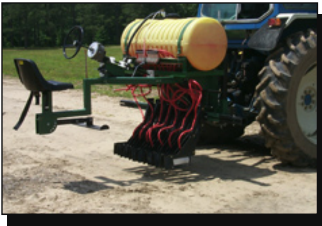
Figure 18—The first-generation MTDC sprayer prototype with fixed-width spray hoods and the original steering wheel.
