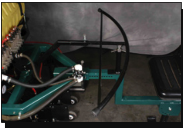
Figure 20—A closeup of the tiller bar used to steer the MTDC Shielded Herbicide Sprayer.
