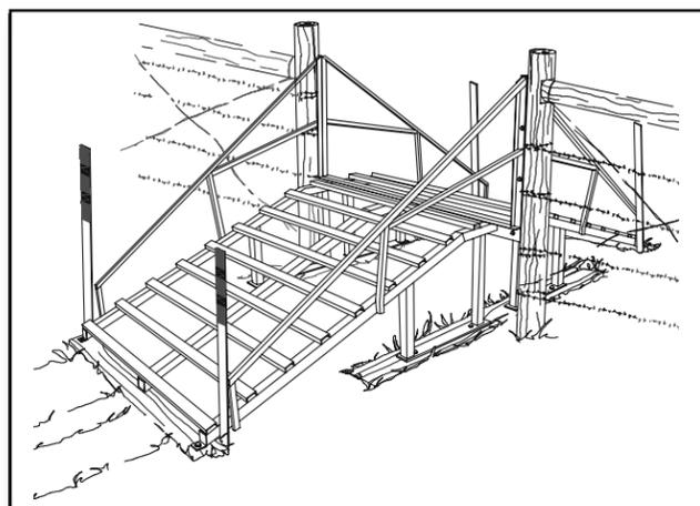
Figure 1—The Southwest Montana ATV Trail Cattle Guard is being used on national forests and BLM public lands in Montana. Object markers may be placed on the center posts instead of on fiberglass stakes at the corners.
