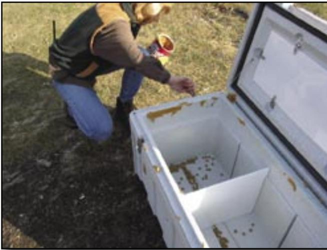
Figure 7—Before containers are tested by captive bears, dog food is placed inside and peanut butter is smeared on seams and latches.
