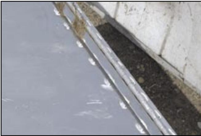
Figures 10b—Although bears broke several welds on the hinge securing the lid of the Bear-Aware Co. prototype storage box, they did not get inside.
