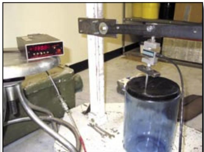
Figure 6—A food-storage container undergoing penetrometer testing at MTDC.
