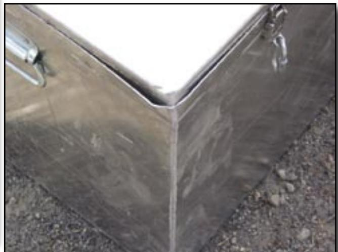
Figures 9b—After 60 minutes, bears slightly damaged the American Whitewater Products prototype insulated dry box.
