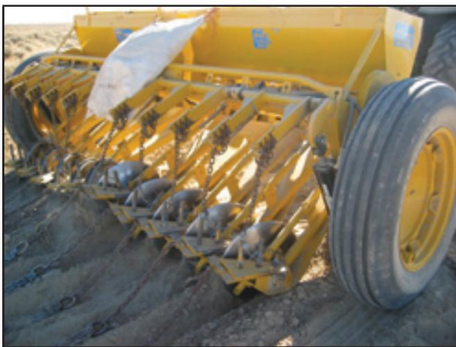
Figure 3—Heavy curved disks clear vegetation and create furrows for the dropped seed. Weight can be added to each disk arm.
