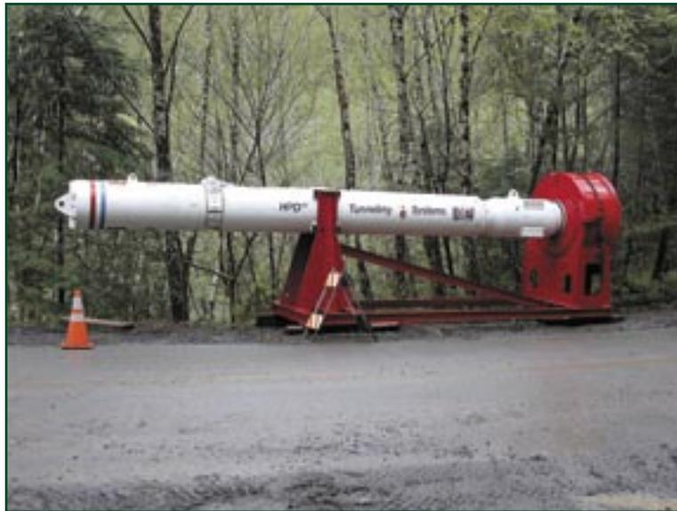
Figure 2—The hammer with red helmet attached to the end.
