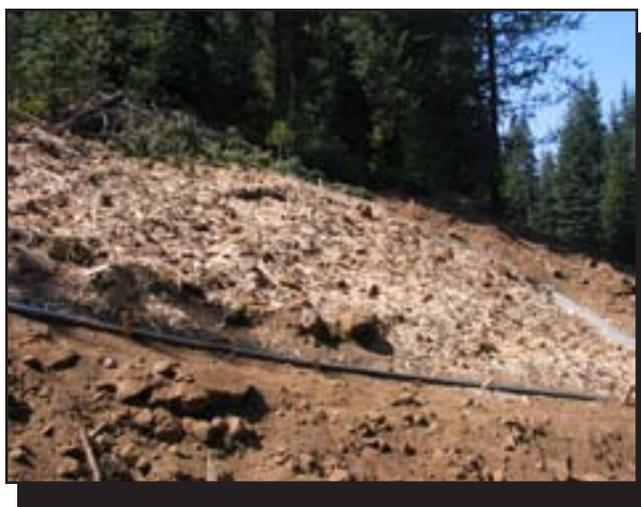
Figure 2—A test plot covered with wood shreadings to reduce erosion.
