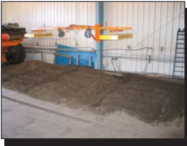
Figure 3—Sandy loam soil being dried and conditioned for testing.
