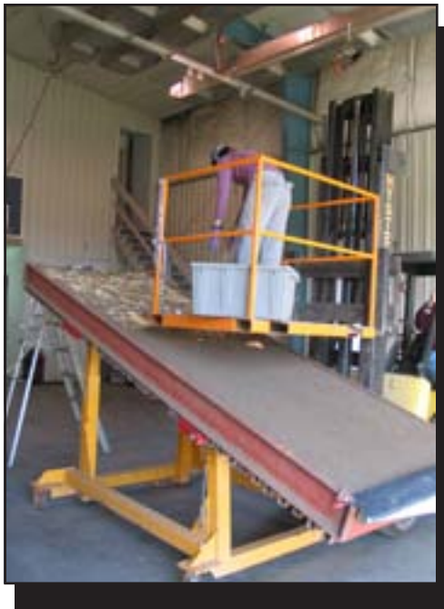
Figure 6—Spreading wood shavings on the soil test plot.
