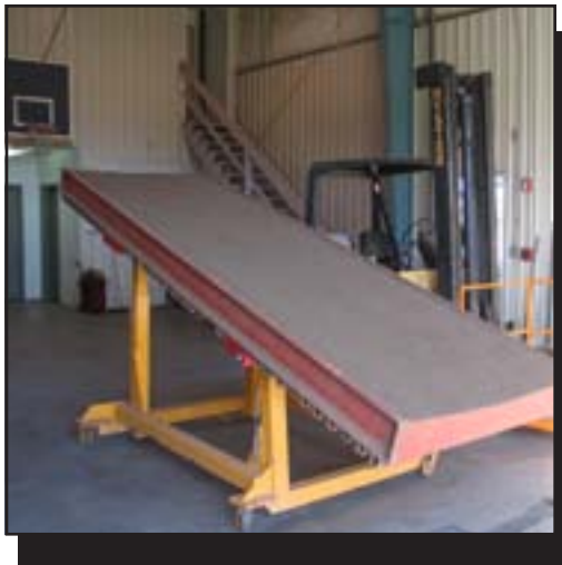
Figure 2—A steel frame with a soil test plot ready for wood shavings.
