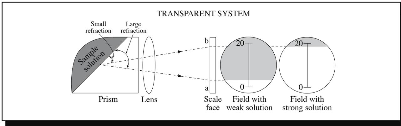
Figure 2—An illustration of the principles used in the transparent detection system of a hand-held refractometer.—Illustration courtesy of ATAGO U.S.A., Inc.
