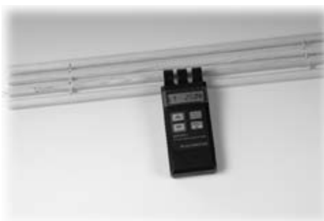
Figure 4—The Holzmeister MoisTest I fuel moisture meter.
