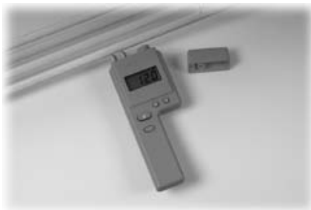
Figure 2—The Delmhorst J-2000 fuel moisture meter.
