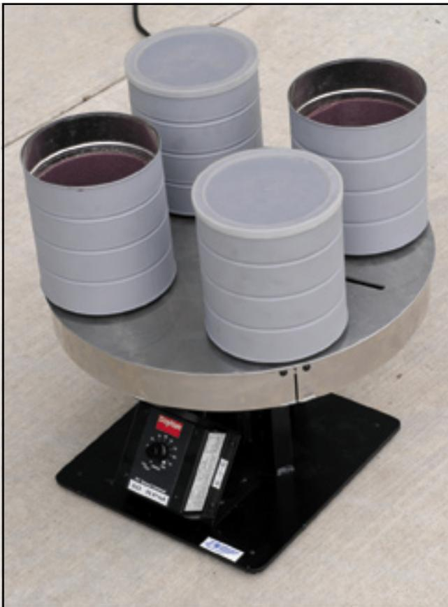
Figure 1—The new sanding scarifier for whitebark pine seed. The seeds swirl across sandpaper lining each of the four cans.
