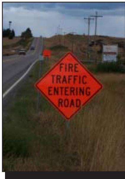
Figure 2—The illustration shows proper sign placement with a warning sign before the guide sign. These signs served a helibase near the Blackfoot Fire in northwestern Montana during 2003.
