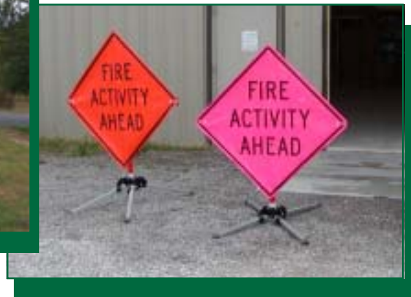
Figure 12—Fluorescent orange signs were compared with new fluorescent pink signs in Northern Region field tests during the 2003 fire season.
