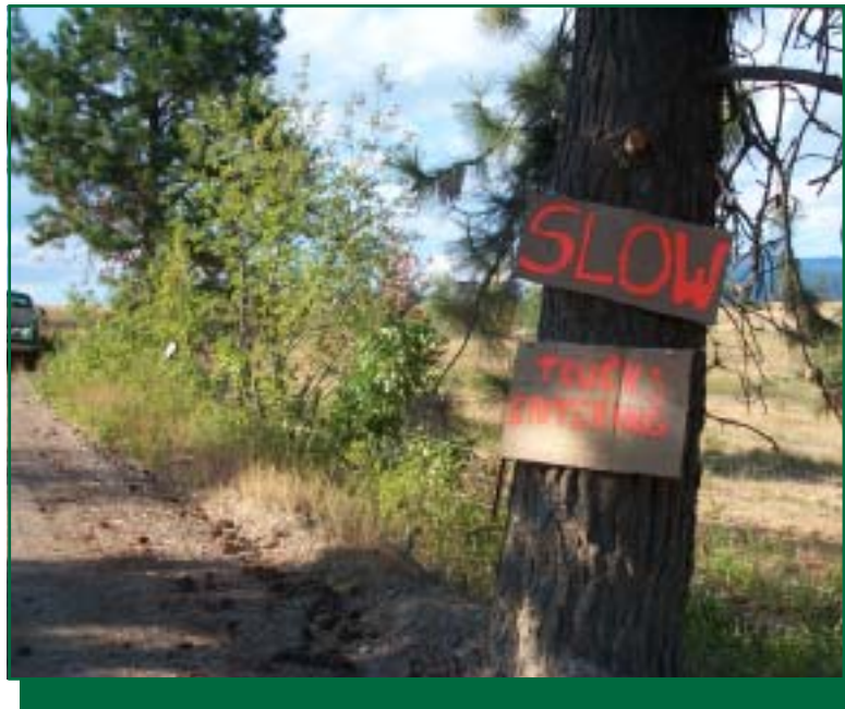
Figure 3—Often signs erected during the early stages of an incident don't provide adequately for the safety of motorists or incident personnel. These signs were at a blind intersection near a helibase serving more than two-dozen helicopters near the Ninemile Fire in western Montana during 2003.
