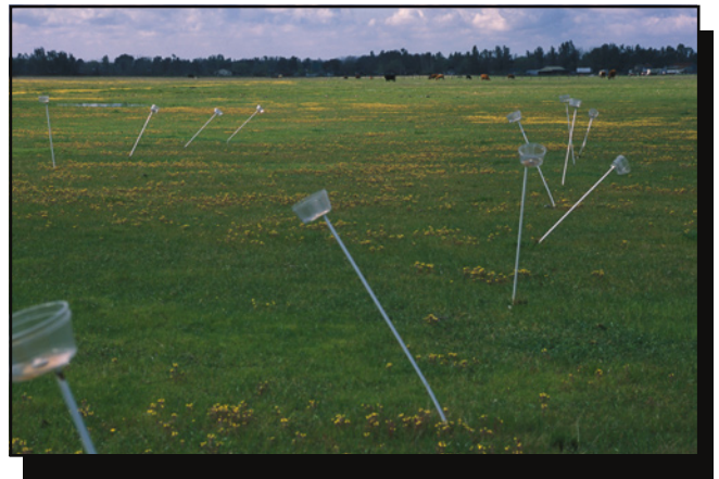
Figure 2—Setup tasks can vary. This grid was overrun by cattle. It took several days to straighten the stakes and replace the cup holders.
