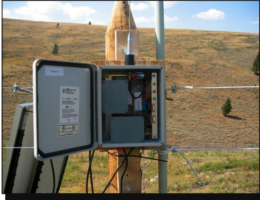
Figure 19—The satellite transmitter sends fence voltage readings hourly, updating a Web page.
