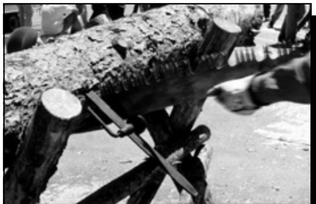
Figure 42—This vintage mechanical underbuck helps hold the saw up so it can cut from beneath the log. This is one design of many that were available.
