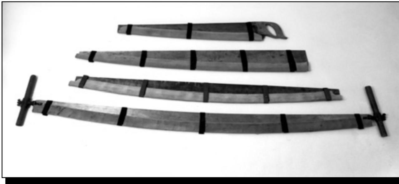
Figure 27—MTDC developed this saw sheath. The guard is made from 1½-inch discarded firehose using nylon straps and hook-and-loop fasteners.
